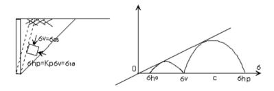
$$Kp = \frac{\sigma_{hp}}{\sigma_v} = \frac{1 + \sin\phi}{1 - \sin\phi} = \tan^2(45^\circ + \frac{\phi}{2}) = \frac{1}{K_a}$$
